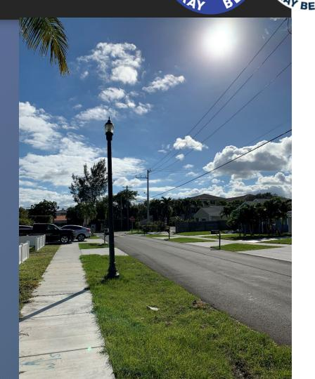
GRANVILLE SERIES LUMINAIRE LEAF STYLE CASTING, FULL COVER AND ROMAN CROSS, 4,900 LUMENS, MULTIVOLT, ROADWAY TYPE 3, 3000K CCT, GREEN GRAY, 20KV/10KA WITH INDUCTIVE FILTER SURGE PROTECTION, 7 PIN PHOTOCONTROL RECEPTACLE AS PER FPL STANDARDS AND AS MANUFACTURED BY HOLOPHANE.
